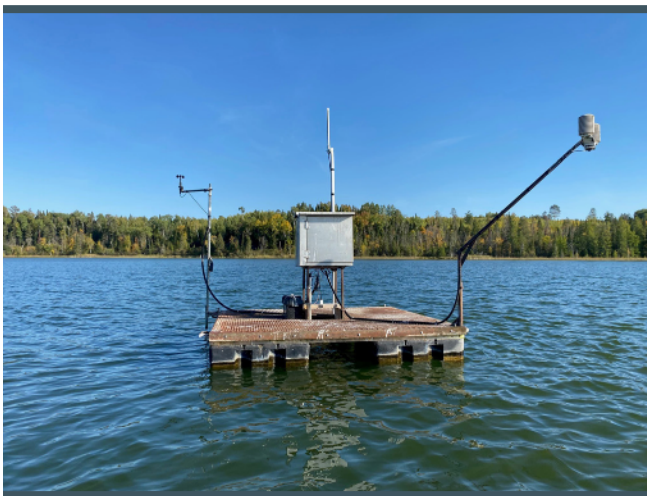
Floating platform with weather and water monitoring equipment at Shingobee Lake. Photo by Carrie Jennings
