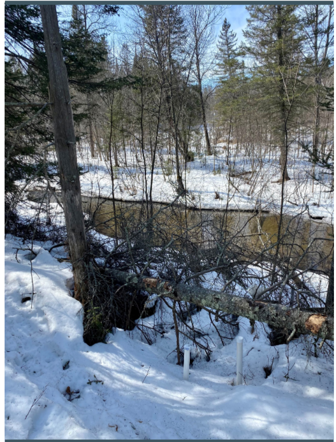
Piezometers measuring groundwater level on hillside as it flows towards the creek discharge area, near Shingobee Lake. Photo by Carrie Jennings
